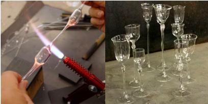
**Lampworking with borosilicate glass**
