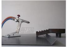
Angle the burner downward when you want to work with a warming station.
